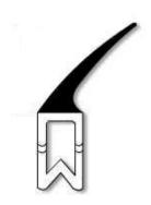
I found a rubber push on gasket that is used as weather stripping around doors. This material is soft rubber with a U channel that will fit over the edge of the catch basin. The U channel contains stainless steel metal clips encased in the rubber that make for a tight fit over any edge. This material can be purchased at automotive parts supply stores I got mine on line in a 25 foot roll.
