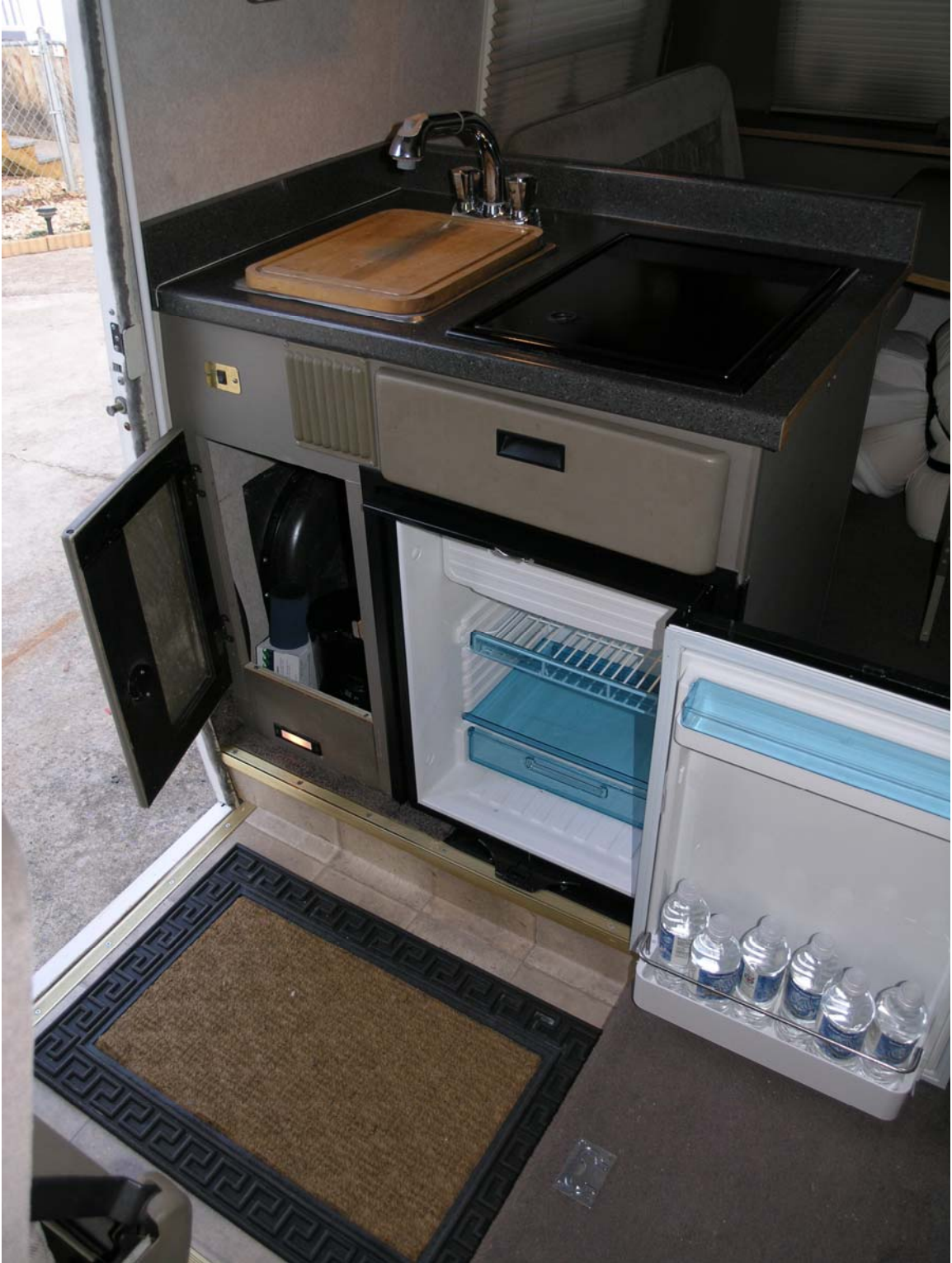
Here you can see the inside of the new door made from the old refrigerator door skin.
