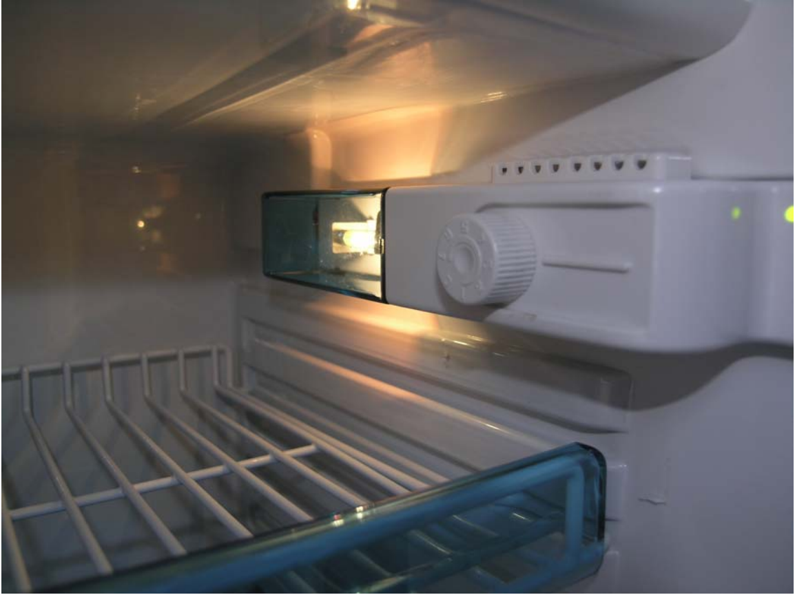
The controls are inside and a green light indicates power on.
