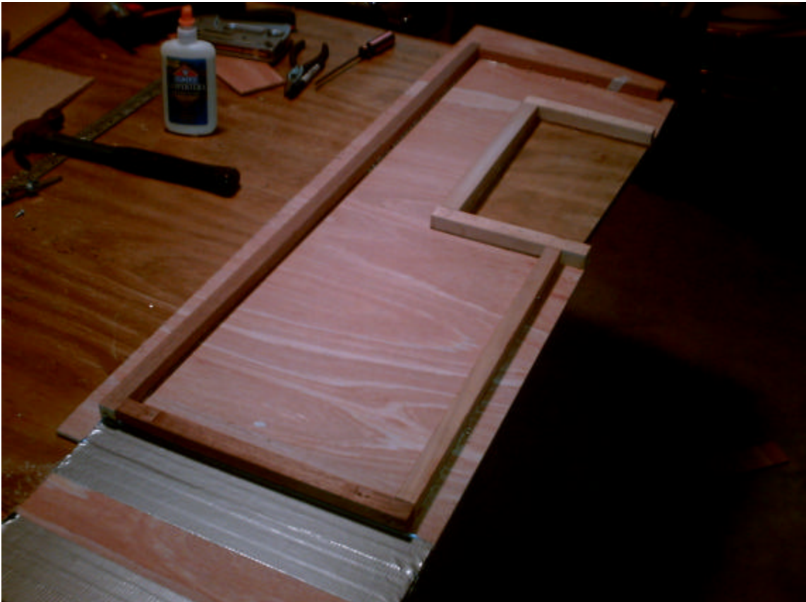
The duck tape forms a hinge for the left side panel. The plywood is much stiffer than the cardboard so it stays in place without the metal clips it just wedges behind the power
