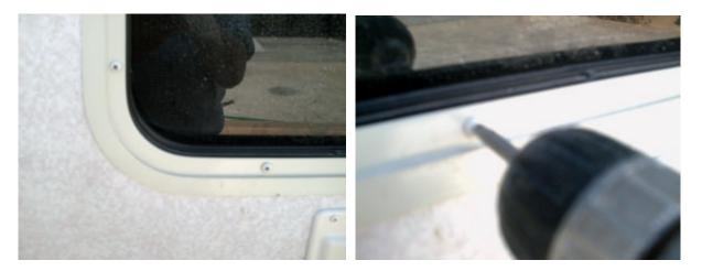
Remove all the screws holding the inside trim ring in place. Then remove the trim ring (it should just fall off after you remove all the screws).
