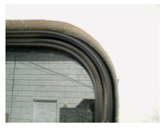
Once you have the frame out clean all the old tape off the lip. If you pull on the tape then use the pieces you get off to stick and pull off more (like removing chewing gum) The cleaning solvent can be used to get the last traces off the frame (it don't have to look like it just came out of the box a little left behind won't hurt).
