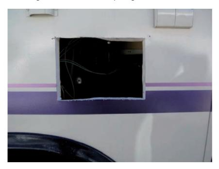
The nice thing about the sawsall is it cuts all the way thru the wall.
