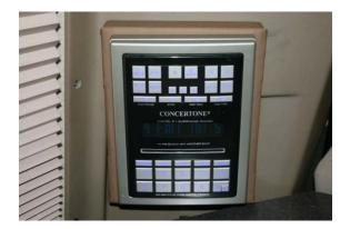
The head unit is mounted into the transition panel behind the driver seat. I had to make a custom trim piece because the area behind the panel was not deep enough for the head unit and all the wiring. There are a zillion wires and connections on the back including power and antenna along with all the speakers and video.
