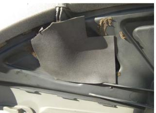
With the dash back in place I reinstalled all the Switches, Steering wheel and the controls. Before I put the vents back in I wanted to repair the foam seals inside them. The vents have flow control flaps inside them that can shut off the air flow to that vent. The control is activated using a sliding knob on the front of each vent. The foam on these control flaps had detoriated and was gone! I used the closed cell art foam to repair these flaps also.
