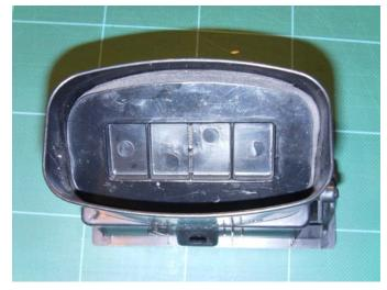
Then pop the flap back into the vent and reconnect the control arm.
