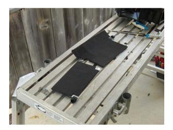
I covered the flaps on both side because they need to seal in both directions also the foam dampens the fan noise. I also put a little grease on the hinge pins to help them move easily.
