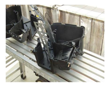
The Air box can be split in two by removing the clips that hold it together and gently pry the halves apart. You can see the metal flaps and the huge holes in them. These should be covered in foam to form a seal where they touch the sides of the box. There are 3 flaps in the box the 2 metal ones and a smaller plastic one that diverts air to the defrosters.
