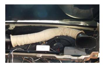
The left and right vent ducts attach to the central vent box. The tubes are insulated with a fabric cover. They just snap in place and can be bent to fit.
