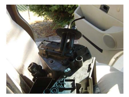
Remove all the vents that attach to the air box and disconnect all the vacuum hoses. You have to disconnect the heater hoses and one vacuum hose at the firewall then lift the air box out of the dash. This will leave a big open space in the dash.
