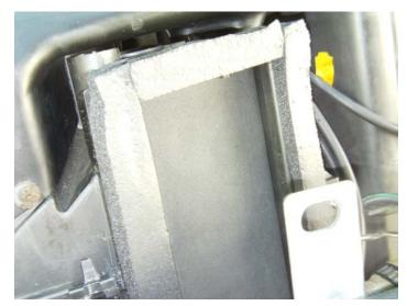
There are 2 main seals under the dash, the one on top goes to the defrosters the other mates with the front vent distrubtion box that is held in with 2 clips.
