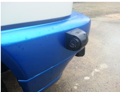
The Right camera mounted to the bumper.
